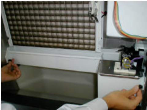
14. By lifting-up a little bit the back of the water reservoir, remove the same from its hook seats.
