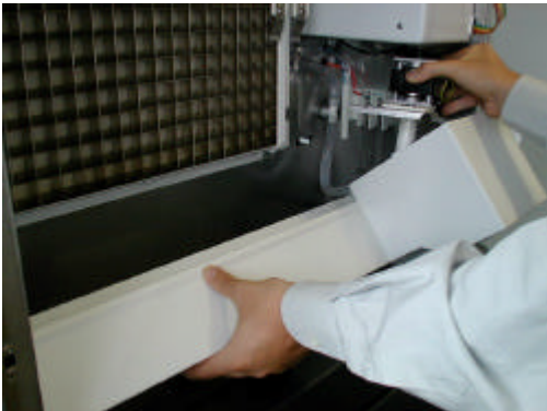
14. By lifting-up a little bit the back of the water reservoir, remove the same from its hook seats.
