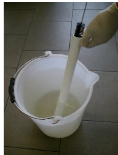
17. ....using different types of brushes clean/sanitize the water distributor tube and .....
