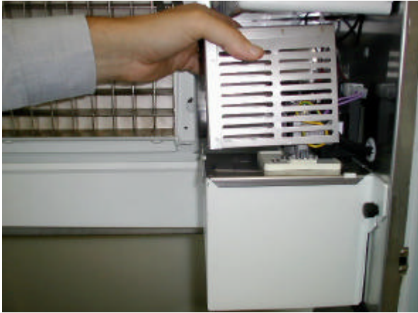
13. Unloose the two screws to remove the water reservoir
